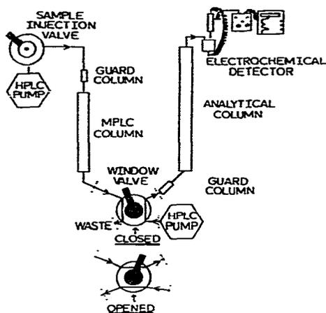
Fig. 1. Window-valve HPLC-EC system. Shown with valve in closed (upper) and opened (lower) positions. Equipment described in text.
